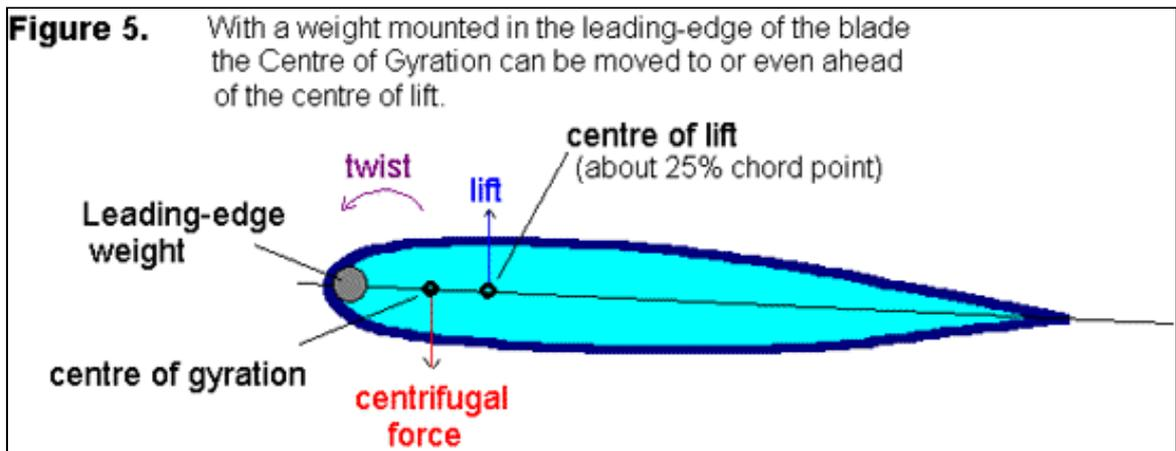
Figure 5 shows the situation when, by the addition of a leading-edge weight, the Centre of Gyration is ahead of the centre of lift. The twist on the blade is now reversed and acts to reduce the angle of attack of the blade. So, any increase in lift will be accompanied by the blade twisting
