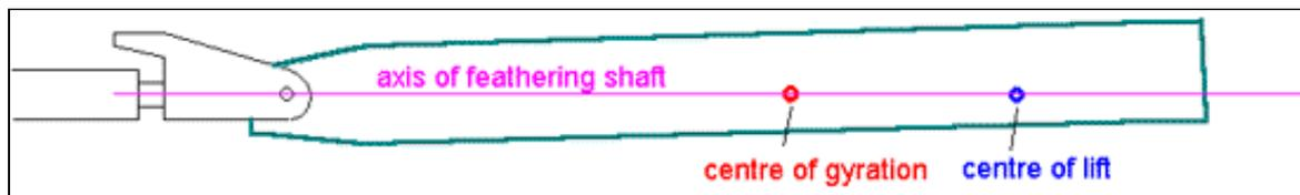
Figure 8. Unweighted blade with bolt hole moved towards trailing edge
