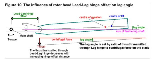
To sum up, the distribution of weight within the blade is important because the combination of a rearward Centre of Gyration and a high degree of torsional flexibility renders the blade susceptible to flutter. However, a very forward Centre of Gyration can cause a high load on the collective servo. This is especially so where a small distance between lead/lag hinges causes large lag angles especially under climb or during high g-load manoeuvres.
