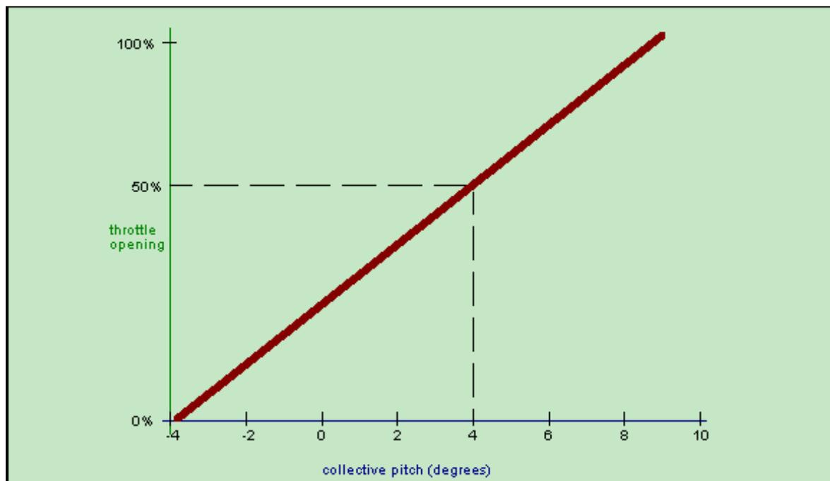
This gives us a basis for a typical 'normal' pitch/throttle curve that will, in level, upright flight give us a substantially constant head RPM as we climb or descend. There are a variety of other arrangements.
