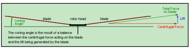
You can see how the forces balance out when the blades are inclined upwards towards the tips by the coning angle. The greater the centrifugal force the smaller the coning angle while the greater the helicopter weight the larger the coning angle. The centrifugal force depends on the weight of the blades, the rotor diameter, and the rotor RPM. How the weight is distributed in the blade is also important. Weight at the ends of the blades has more effect than weight near the root.
