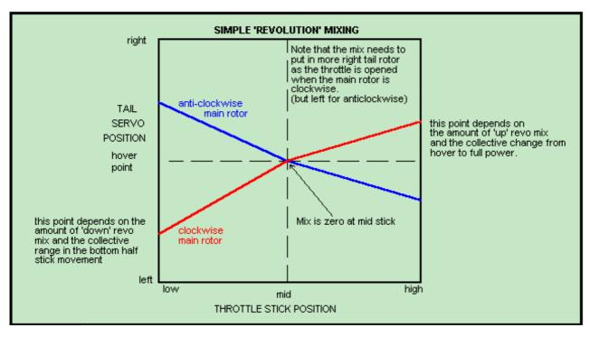
In 'normal' pitch range the tail rotor pitch needs to reduce as the throttle is closed (and the collective pitch is lowered). A fairly obvious point here is that when the throttle is closed to tickover (or at least to the point at which the clutch disengages) the engine will be applying no torque to the main rotor so the tail rotor pitch should be zero.
