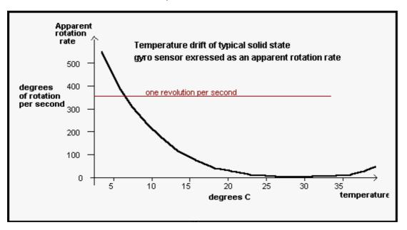
At low temperatures especially this drift is severe. If the sensor is zeroed at 10 degrees C and then cools by only 1 degree C its output will change by the equivalent of a rotation rate of about 30 degrees per second. Since the gyro sensor is otherwise 'blind' it can't tell the difference between output changes due to yaw rates and output changes due to temperature changes.
