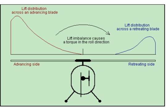
Even at a modest advance ratio of 0.3 about 80% of the lift would be generated on the advancing side of the rotor. This lift imbalance would cause a torque (turning effort) in the roll direction, but because of gyroscopic effects would result mainly in a nose up pitching of the helicopter.
