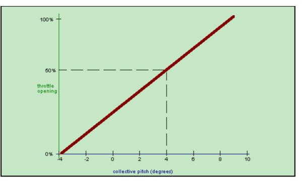
This gives us a basis for a typical 'normal' pitch/throttle curve that will, in level, upright flight give us a substantially constant head RPM as we climb or descend. There are a variety of other arrangements.
