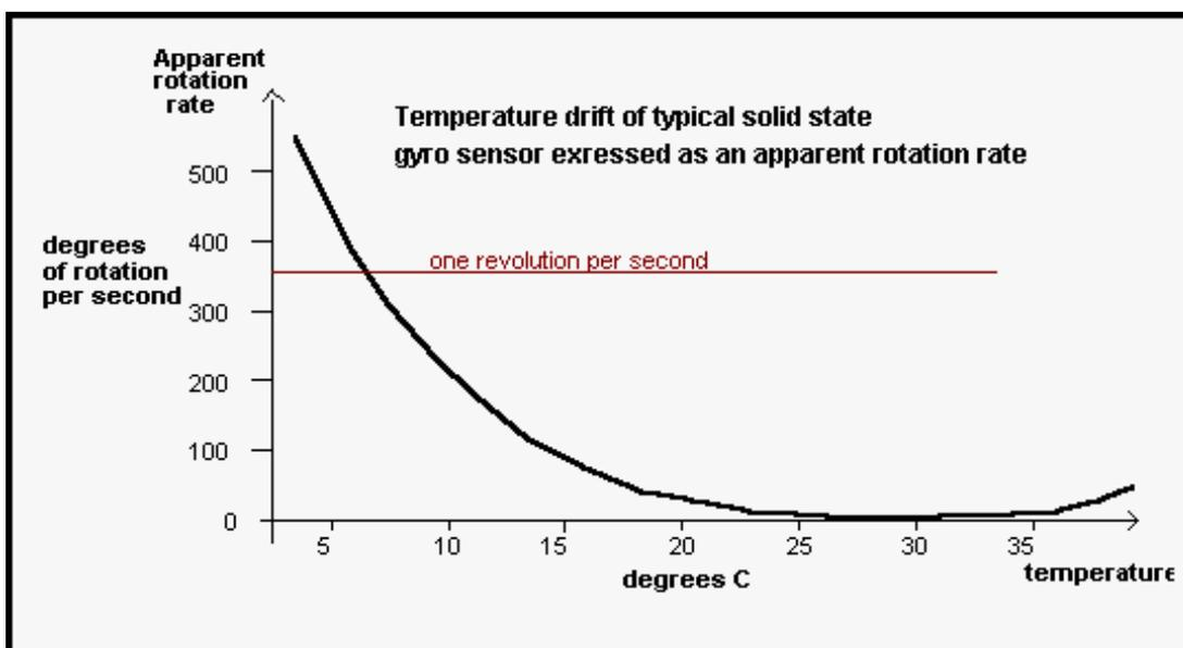
At low temperatures especially this drift is severe. If the sensor is zeroed at 10 degrees C and then cools by only 1 degree C its output will change by the equivalent of a rotation rate of about 30 degrees per second. Since the gyro sensor is otherwise 'blind' it can't tell the difference between output changes due to yaw rates and output changes due to temperature changes.
