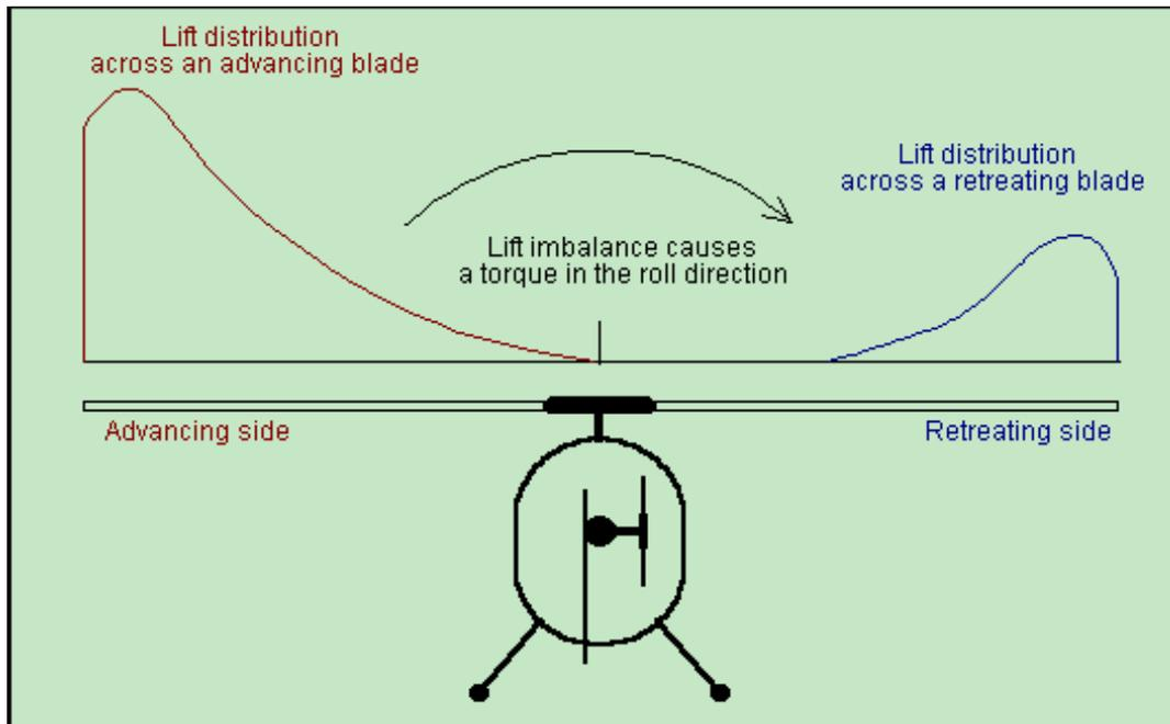
Even at a modest advance ratio of 0.3 about 80% of the lift would be generated on the advancing side of the rotor. This lift imbalance would cause a torque (turning effort) in the roll direction, but because of gyroscopic effects would result mainly in a nose up pitching of the helicopter.
