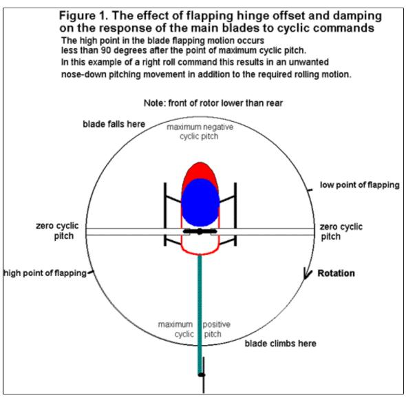
In this illustration we see what happens if we continue to apply the cyclic controls 90 degrees ahead of the required motion. Notice how the right roll command now additionally causes a nose down pitching motion. To combat this the control system needs to feed the cyclic inputs in later in the rotation. This can be done by rotating the swash plate in the direction of rotation. With the cyclic controls retarded in this way the correct response to cyclic inputs is obtained as seen below.
