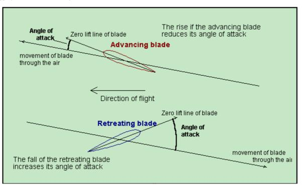
The vertical motion of the blades reduces the angle of attack where the blade is rising (on the advancing side) while increasing it where the blade is falling. When the blades are free to flap these changes in angle of attack occur naturally and need no special geometry of the head. These cyclic attack angle changes result in lift coefficient changes that eliminate the imbalance in lift between the advancing and retreating sides.
