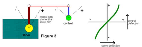
Conversely, a control arm shorter than the servo arm moves through a bigger angle than the servo with an increasing sensitivity towards the ends of the servo travel (see figure 3).
