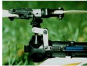
*Here the bellcrank angle has been dictated by the need to clear the sideframe. Unfortunately, to get the pushrod to the servo at the right angle to this bellcrank it needs to be attached directly to the output shaft without any arm at all. This give perfect linearity but leaves the pitch range woefully short.*
