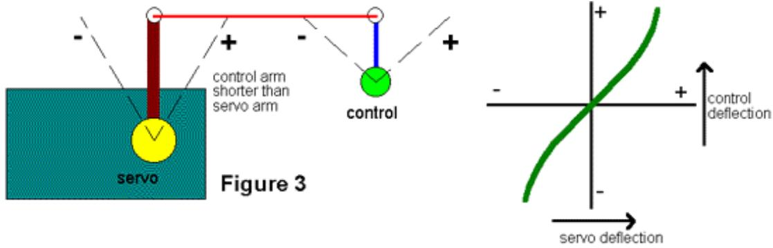
Conversely, a control arm shorter than the servo arm moves through a bigger angle than the servo with an increasing sensitivity towards the ends of the servo travel (see figure 3).
