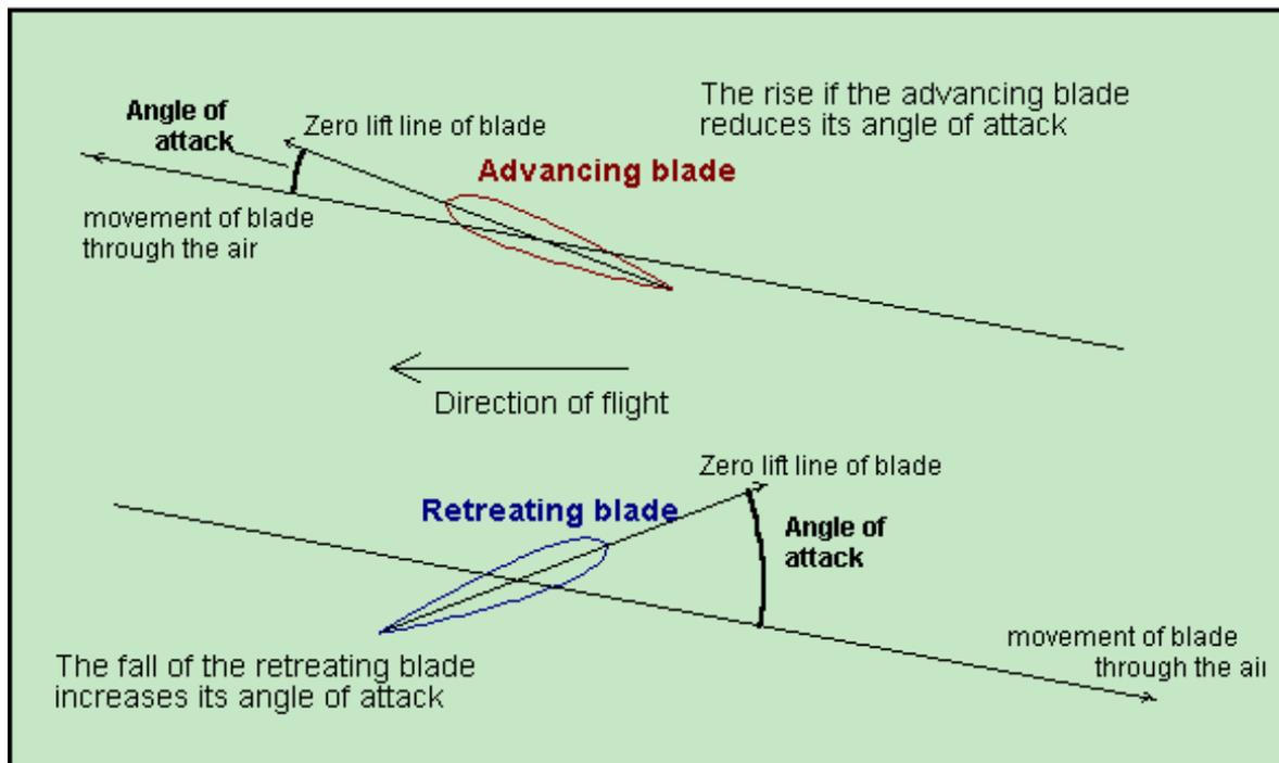
The vertical motion of the blades reduces the angle of attack where the blade is rising (on the advancing side) while increasing it where the blade is falling. When the blades are free to flap these changes in angle of attack occur naturally and need no special geometry of the head. These cyclic attack angle changes result in lift coefficient changes that eliminate the imbalance in lift between the advancing and retreating sides.
