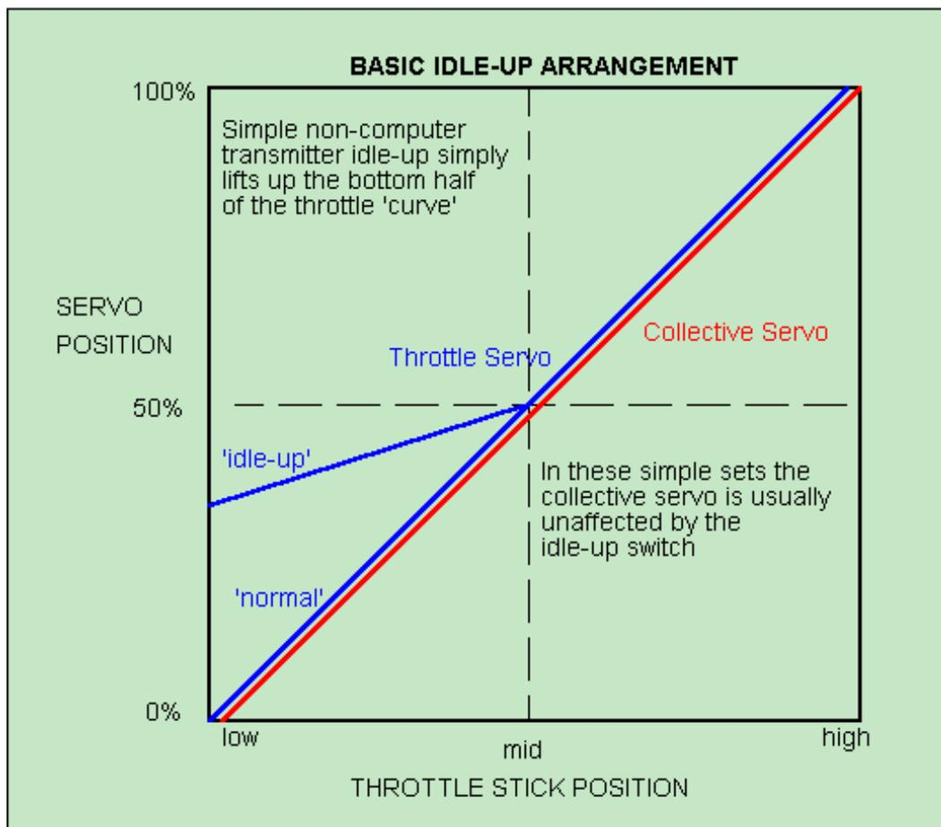
The name comes from the facility on early basic heli transmitters in which a switch on the set allowed the minimum throttle opening (with the throttle stick at the idle position) to be increased - hence the name 'Idle Up'. At certain times (such as the inverted bit of a roll
