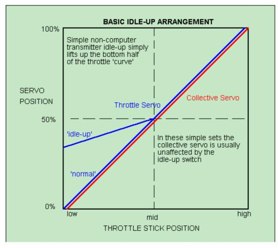
The name comes from the facility on early basic heli transmitters in which a switch on the set allowed the minimum throttle opening (with the throttle stick at the idle position) to be increased - hence the name 'Idle Up'. At certain times (such as the inverted bit of a roll http://www.lance.co.uk/w3mh/articles/html/csm3\_4.htm
