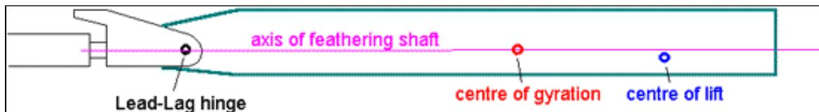
Figure 6. Unweighted blade with bolt hole in line with centre of gyration
