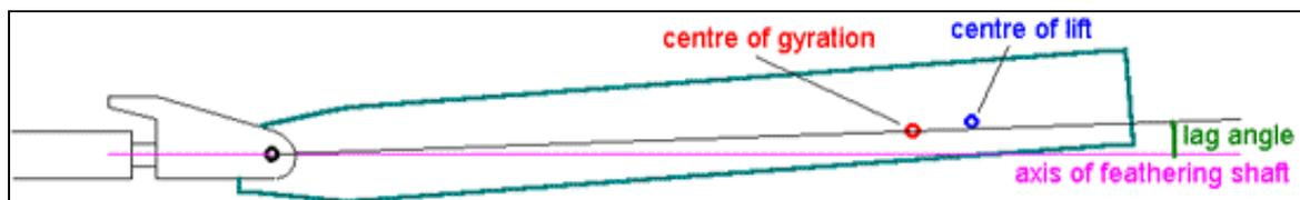
Figure 9. Effect of lag angle on the distance between feathering shaft axis and centre of lift.
