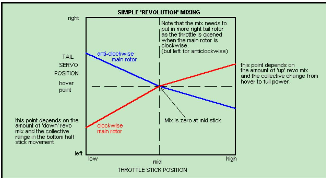
In 'normal' pitch range the tail rotor pitch needs to reduce as the throttle is closed (and the collective pitch is lowered). A fairly obvious point here is that when the throttle is closed to tickover (or at least to the point at which the clutch disengages) the engine will be applying no torque to the main rotor so the tail rotor pitch should be zero.
