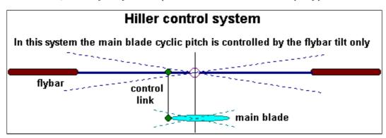
The amount of cyclic control applied to the main blades is automatically adjusted so that the correct roll rate is maintained. The more the main rotor lag behind the flybar the greater the cyclic control applied to the main blades and vice versa.
