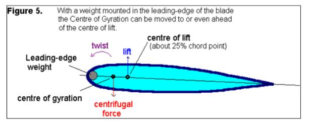
Figure 5 shows the situation when, by the addition of a leading-edge weight, the Centre of Gyration is ahead of the centre of lift. The twist on the blade is now reversed and acts to reduce the angle of attack of the blade. So, any increase in lift will be accompanied by the blade twisting
