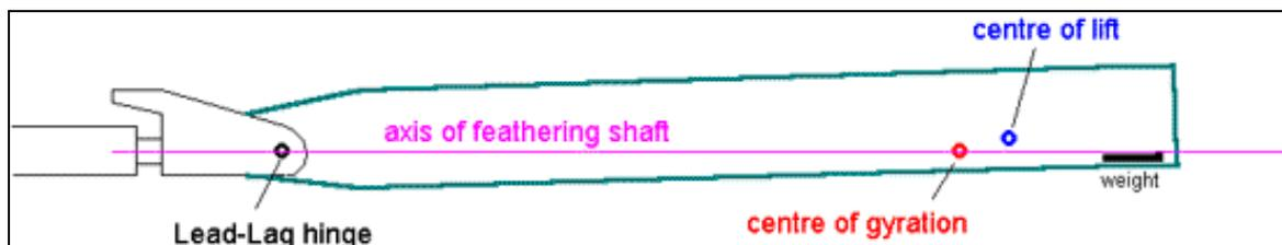
Figure 7. Blade with leading edge weight towards tip
