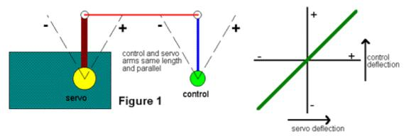
In this case the angular deflection of the control accurately matches that of the servo however, any other arrangement introduces non-linearity into the control movement.
