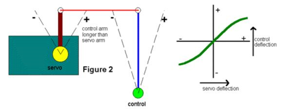
In figure 2 we have a control arm that is longer than the servo arm. If course, the angular movement of the control is now less than that of the servo but the sensitivity of the control movement falls off near the extremes of movement.
