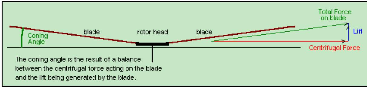
You can see how the forces balance out when the blades are inclined upwards towards the tips by the coning angle. The greater the centrifugal force the smaller the coning angle while the greater the helicopter weight the larger the coning angle. The centrifugal force depends on the weight of the blades, the rotor diameter, and the rotor RPM. How the weight is distributed in the blade is also important. Weight at the ends of the blades has more effect than weight near the root.
