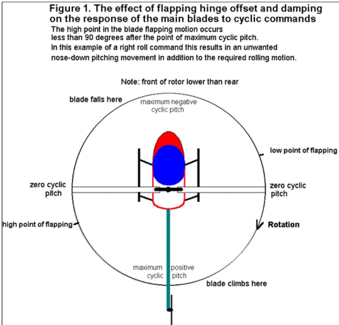
In this illustration we see what happens if we continue to apply the cyclic controls 90 degrees ahead of the required motion. Notice how the right roll command now additionally causes a nose down pitching motion. To combat this the control system needs to feed the cyclic inputs in later in the rotation. This can be done by rotating the swash plate in the direction of rotation. With the cyclic controls retarded in this way the correct response to cyclic inputs is obtained as seen below.
