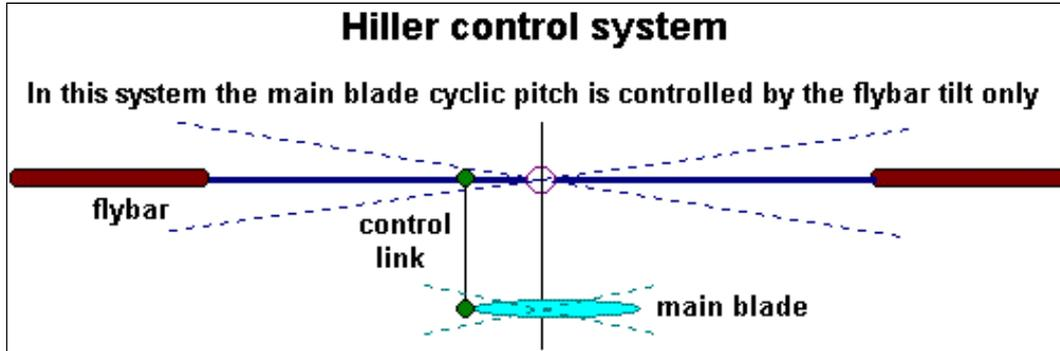
The amount of cyclic control applied to the main blades is automatically adjusted so that the correct roll rate is maintained. The more the main rotor lag behind the flybar the greater the cyclic control applied to the main blades and vice versa.
