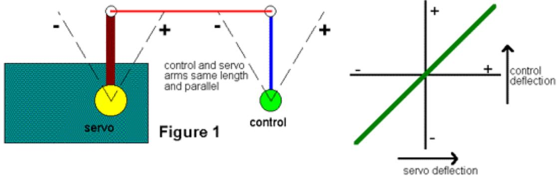
In this case the angular deflection of the control accurately matches that of the servo however, any other arrangement introduces non-linearity into the control movement.
